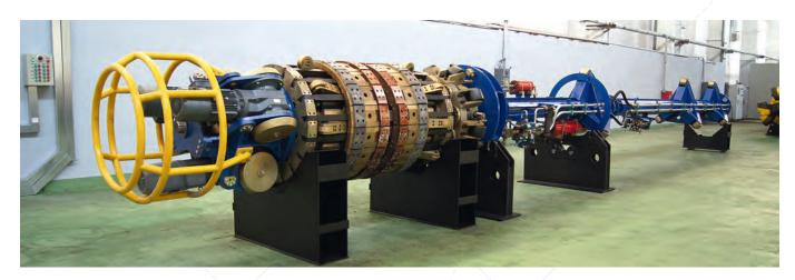
**Land equipment complexes KCC-01, KCC-04** are designed for FBW of pipes of large diameters. The machines are used for construction of oil and gas pipelines from steels of different hardness groups up to K65 (X80).
